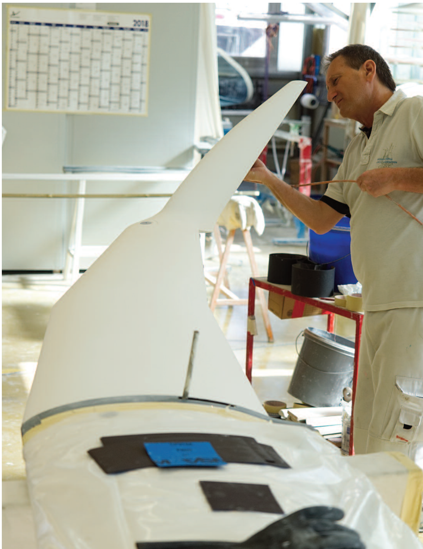
Fitting of the 15m tips on the existing main wing part of "F2", SHK paintshop
