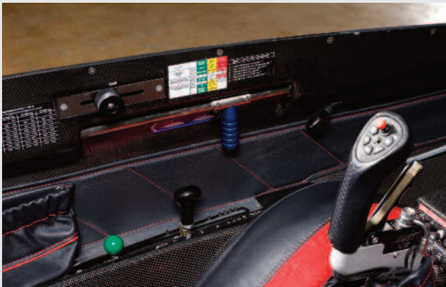
Left cockpit side with controls and new TOST brake
