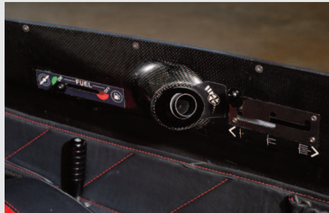
Right cockpit side with vent, ballast and gas openers
