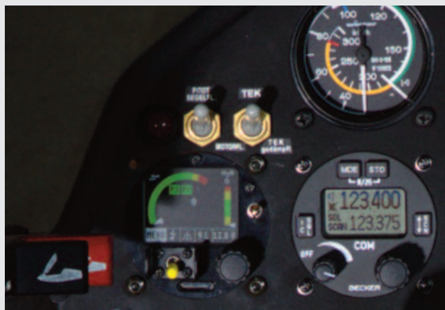
New modern ILEC engine management controller
